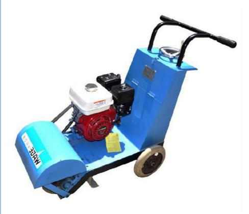
HGQ Pavement sweeping machine is mainly used in cleaning the cement floating slurry, mud and dust on the road surface, the gasoline engine would drive the steel wire brash to grind the road surface for cleaning work. The machine frame is equipped with a sweeping strength adjuster, we can adjust the sweeping strength according to the real situation, it can save time, labor, and improve working efficiency.
