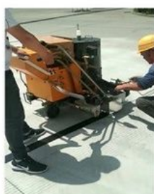
Thermoplastic road marking machine
