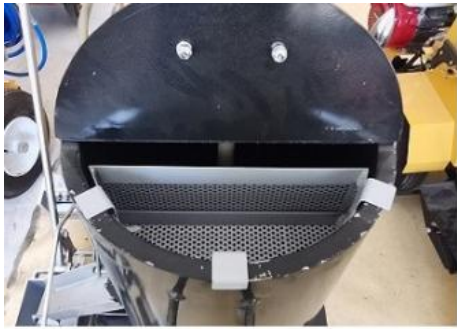
Paint Tank & Filter
