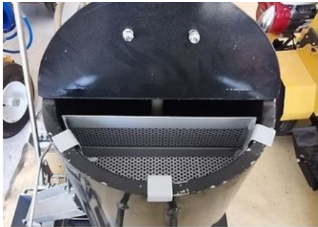
Paint Tank & Filter
